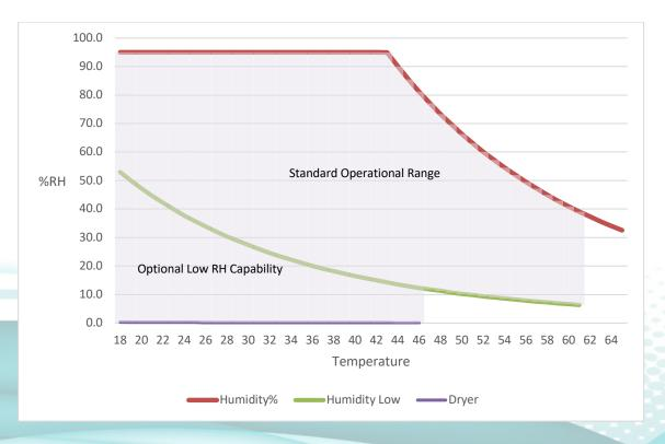
Humidity% represents chamber performing at 42°C Dew point. Humidity Low represents absolute humidity at ambient space of 23°C and 50%RH.
