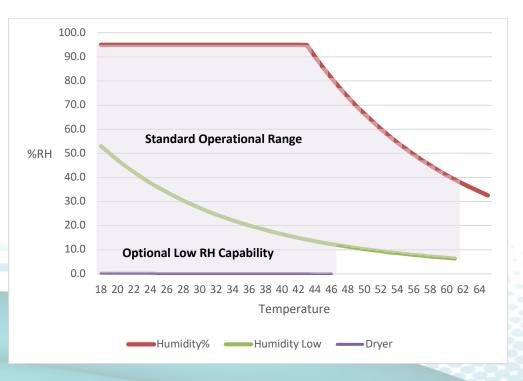
Humidity% represents chamber performing at 42°C Dew point. Humidity Low represents absolute humidity at ambient space of 23°C and 50%RH.
